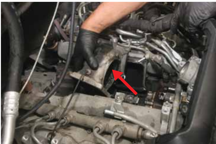
STEP 23 Remove intake manifold bridge Now with all components removed from engine you can start assembly of 4094 turbo.
