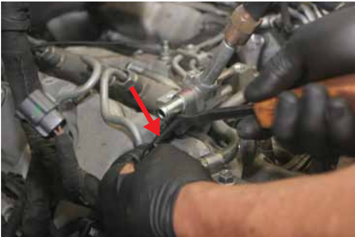
STEP 21 Remove passenger side fuel return.
