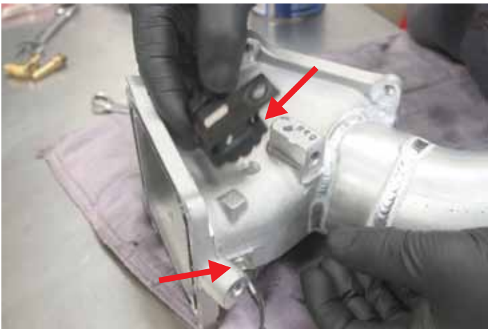
STEP 28 Install M.A.P. sensor and intake temperature probe on new intake manifold bridge.
