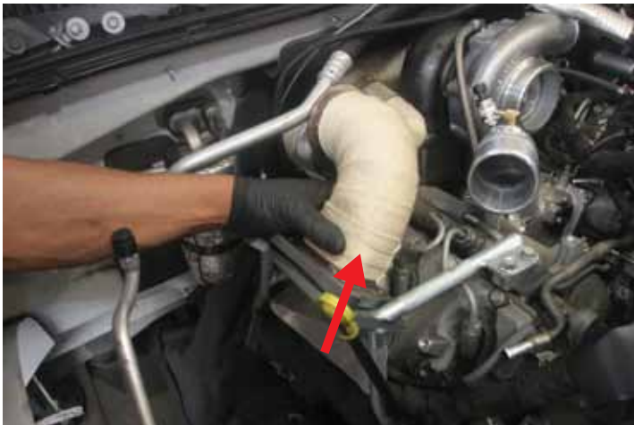
STEP 47 Install waste gated exhaust tube with gasket.
