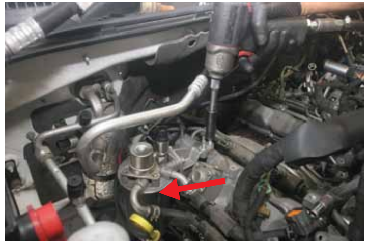
STEP 20 Remove fuel filter/ fuel filter bracket.
