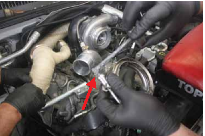
STEP 48 Put anti seize on all exhaust clamps.
