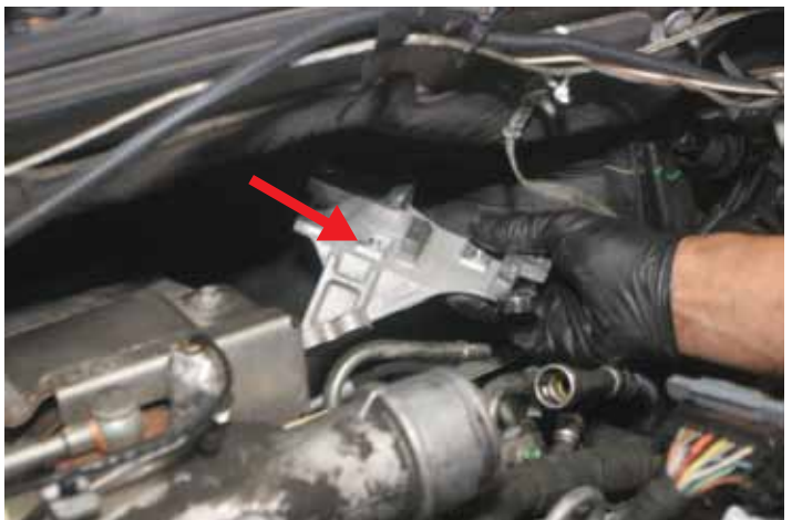
STEP 15 Remove glow plug control module and mounting bracket.
