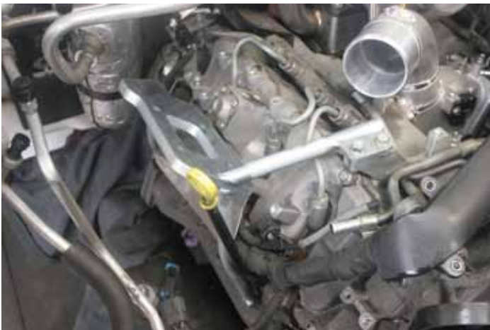
STEP 41 Install turbo mounting bracket.
