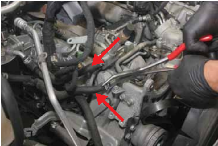
STEP 19 Remove fuel lines.
