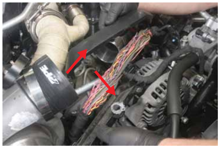
STEP 55 Remove plastic protector from wiring loom and rewrap with electrical tape.
