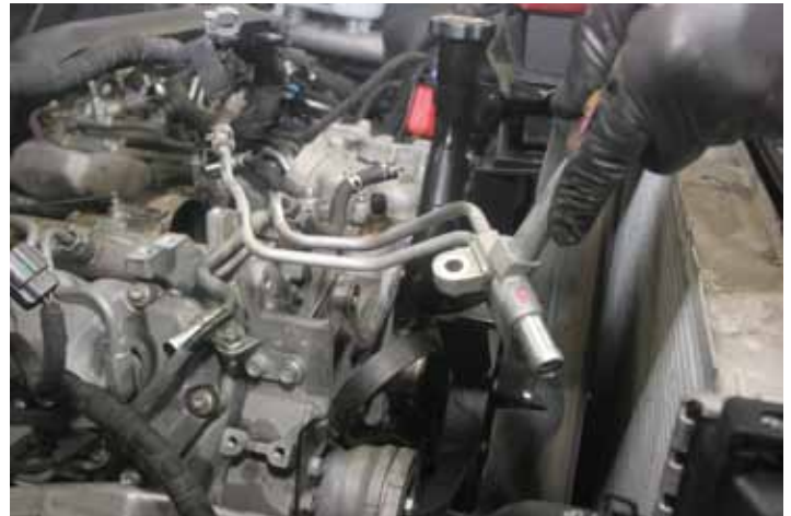
STEP 22 Remove fuel pressure valve assembly.
