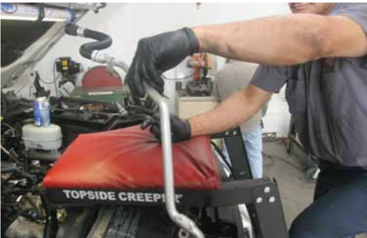
STEP 9 Remove heater lines.
