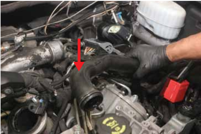
STEP 12 Remove coolant tube.
