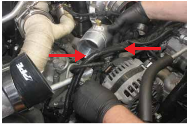
STEP 56 Push wrapped harness down behind alternator. Reconnect all wiring connections. Prepare wastegate for installation.
