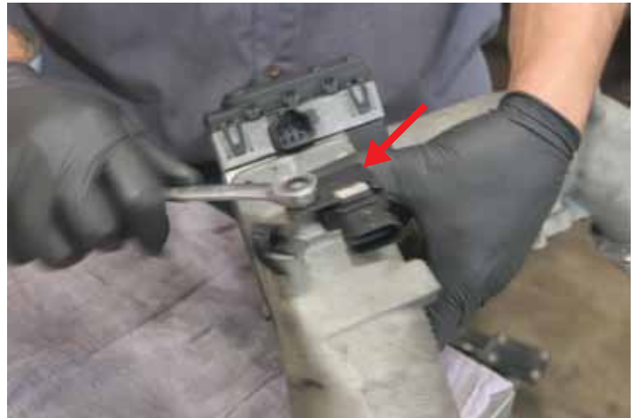
STEP 27 Remove M.A.P. sensor from intake.
