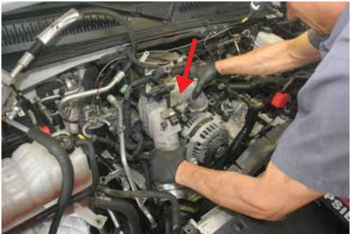
STEP 7 Remove air intake.
