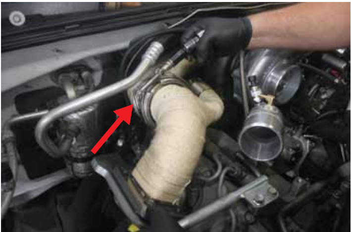
STEP 49 Loosely install clamps.
