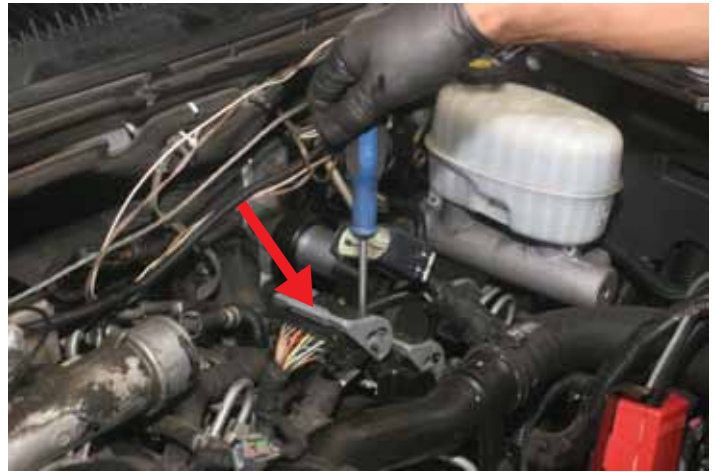
STEP 11 Remove engine harness bracket.
