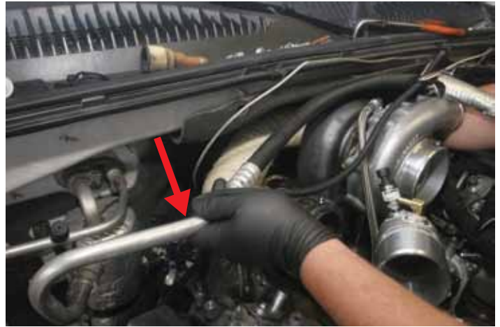
STEP 46 Slightly bend the AC line up to allow clearance for pipe.
