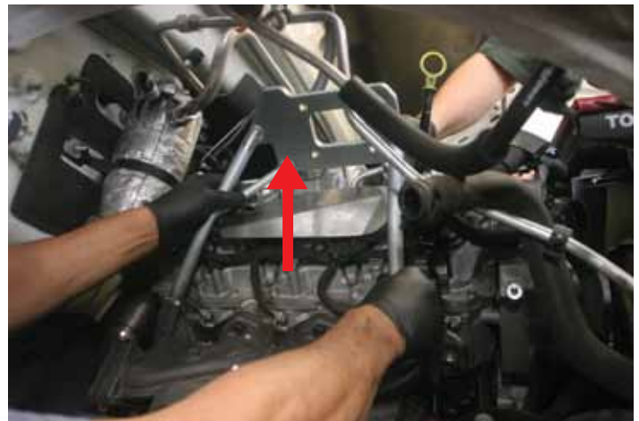
STEP 40 Install turbo mounting bracket.
