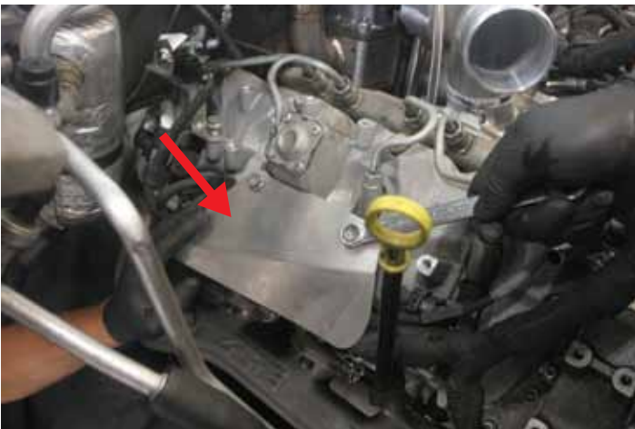
STEP 39 Install aluminum heat shield.
