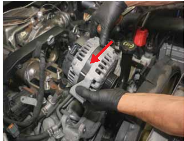
STEP 8 Remove alternator.
