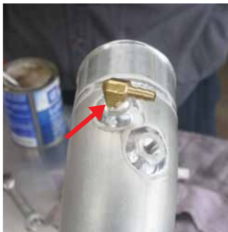
STEP 29 Install brass fitting using Teflon tape, fitting should face rearward, second port is for boost gauge.
