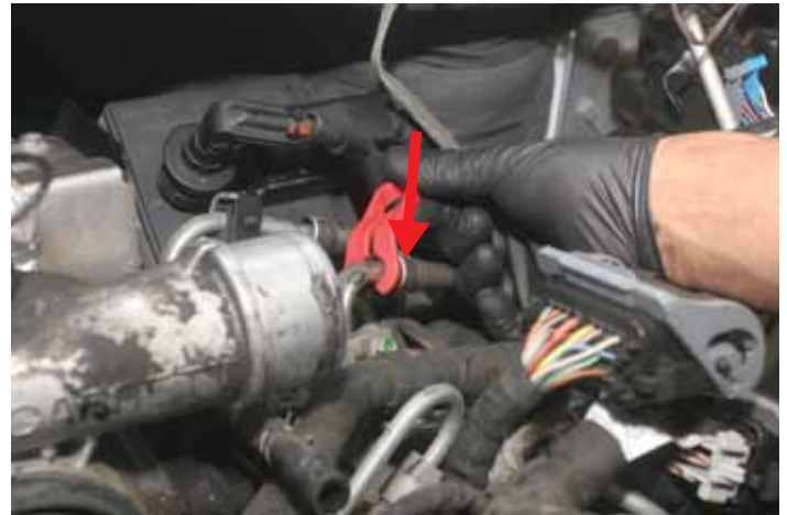
STEP 13 Remove fuel lines.
