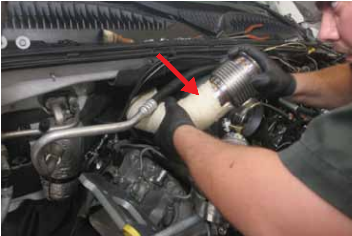
STEP 45 Install 3" exhaust pipe after it has been wrapped.
