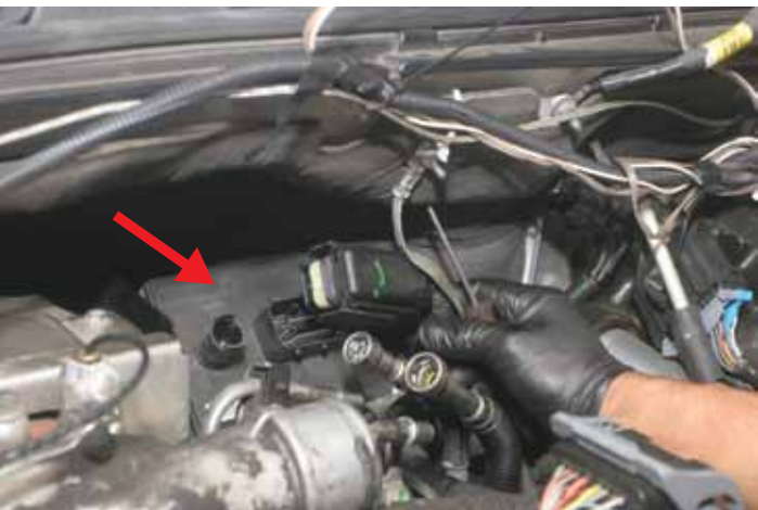
STEP 14 Remove glow plug control module and mounting bracket.
