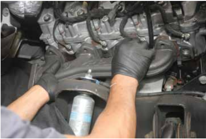
STEP 38 Install new exhaust up-pipes and manifolds.
