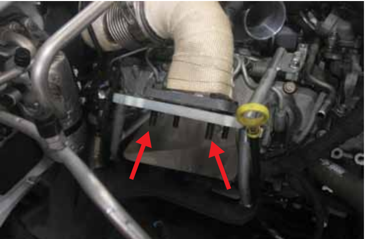
STEP 50 Place bolts in flange. Install turbo gasket.
