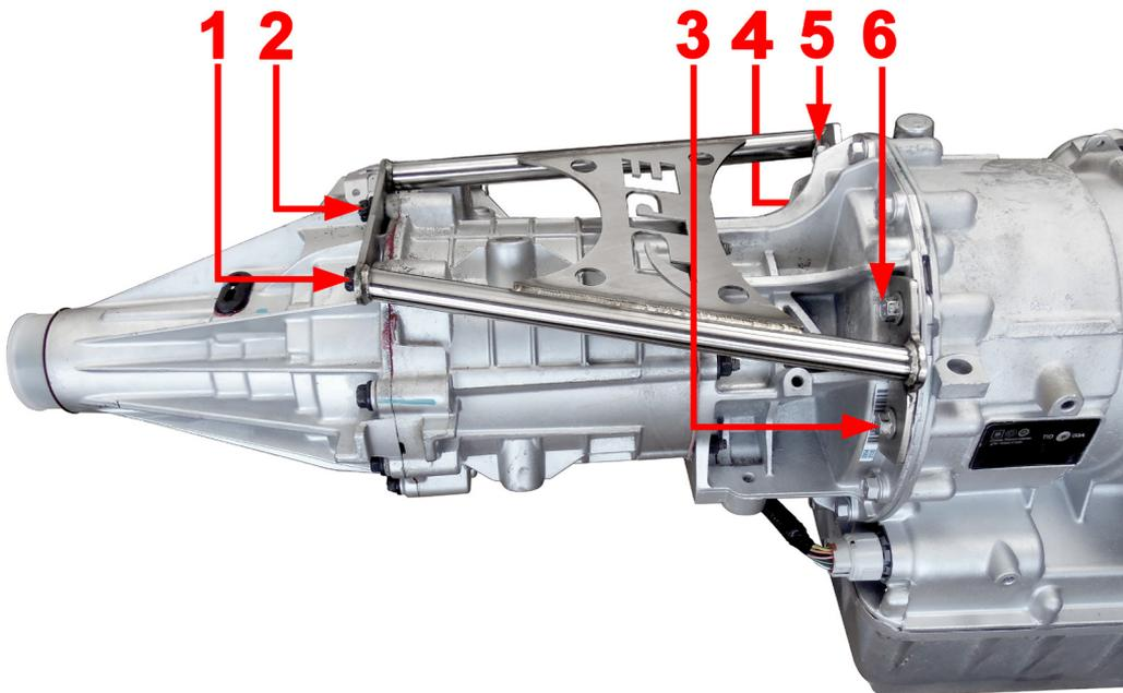
**Step 2:** *Place Transfer Case Brace in position and install factory bolts.*
