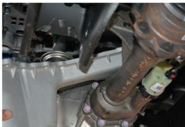
*Once in position, install two factory bolts on each side (middle) to secure the pan. Finger-tighten bolts to hold pan in position.*
