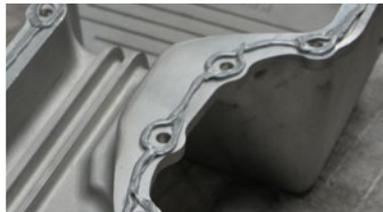
**Step 9.** *It is very important not to smear the sealant while installing the new pan. It is recommended you have help in locating the dowel pin, which indexes the pan in the proper position.*
