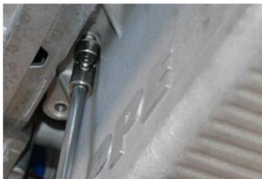
**Step 11.** *Check and mark bell housing bolt for trimming. Use a cut-off wheel to trim excess. Reinstall bolt and torque to manufacturer spec.*
